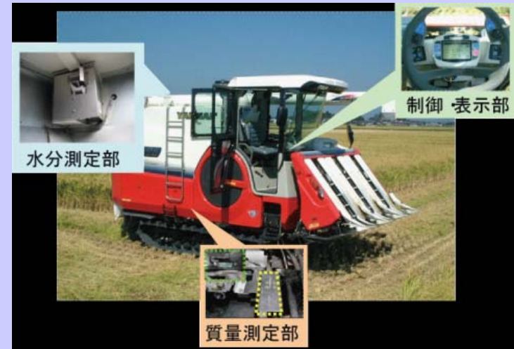
Harvester equipped with yield sensor
