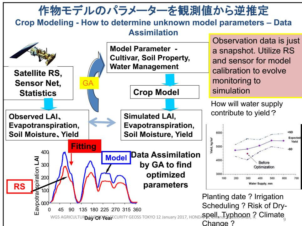
Comparison of Satellite LAI and Simulated LAI
