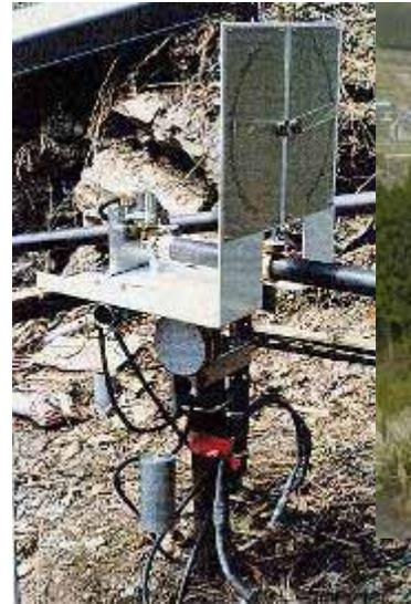
3-D shear displacement meters
