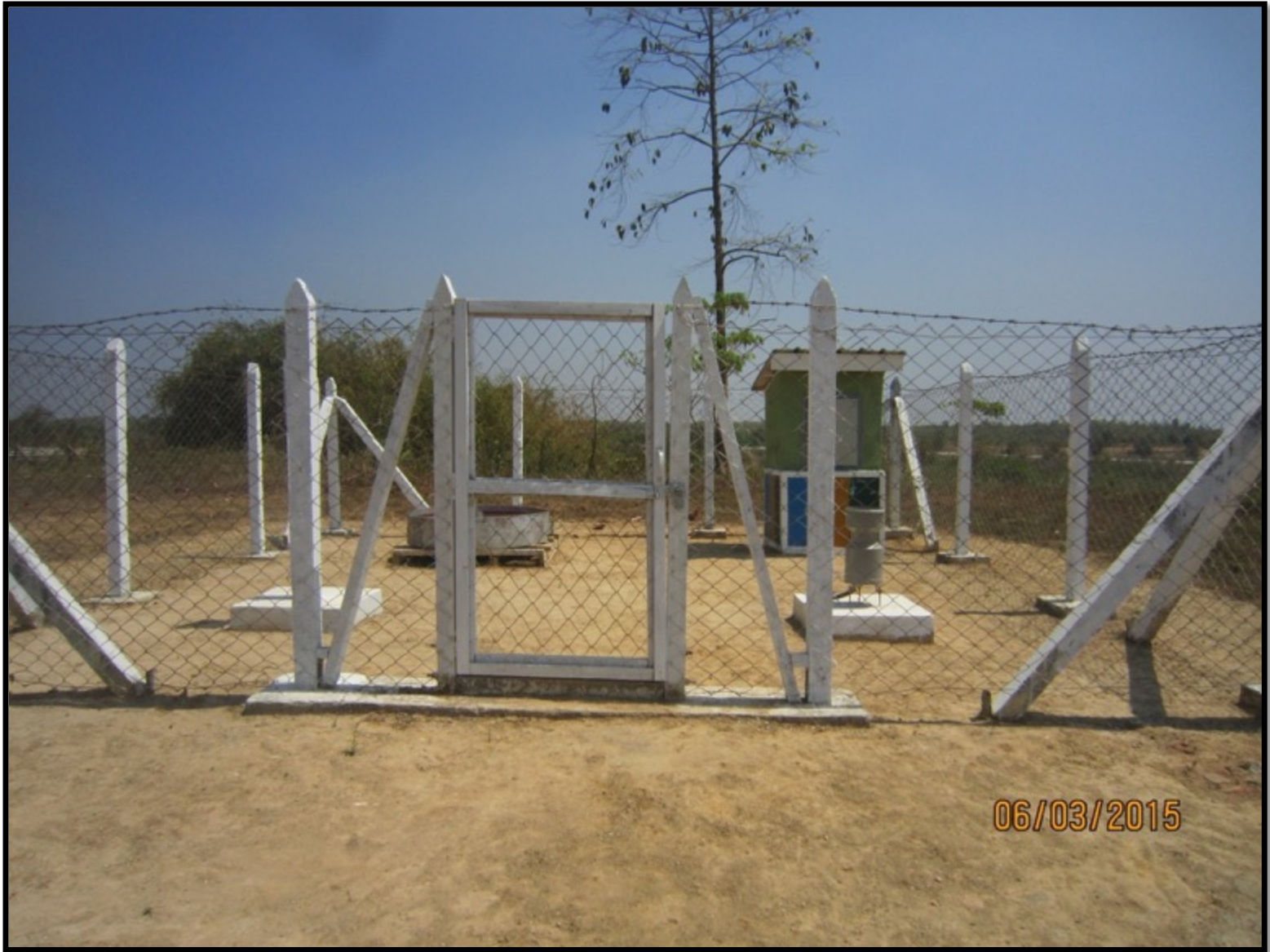
Auto Rain gauge Station at Wakadoke Dam
