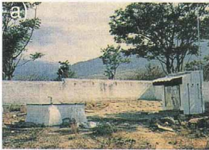
Figure 3. Site condition at a) PCI station and b) PPI station. A small building to install data logger and a roof of the seismic vault are seen. A solar cell is installed on the top of the building. GPS is installed on the top of a pole.
